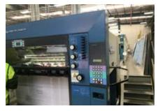
Our multi-colour offset printing presses can apply speciality finishing, such as UV varnish, in-line with a printed sheet size up to 1020 x 1420mm.
