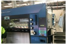
Our multi-colour offset printing presses can apply speciality finishing, such as UV varnish, in-line with a printed sheet size up to  $1020 \times 1420$ mm.
