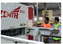
Our die-cutting capabilities are second to none; we can either flat-bed die-cut to a massive 1650 x 2500mm or high speed rotary cut to 1575 x 2800mm.
