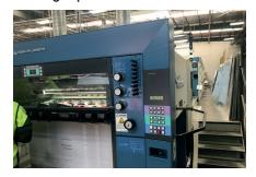
Our multi-colour offset printing presses can apply speciality finishing, such as UV varnish, in-line with a printed sheet size up to  $1020 \times 1420$ mm.
