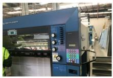
Our offset printing presses are multi-colour and can apply speciality finishing like UV varnish, in line with a printed sheet size capability of 1020 x 1420mm.
